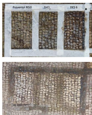
Fig. 2. Application of DES 6 (above) and after application (below) in area of the mosaic in the Archeological Park of Ostia Antica (Rome).
