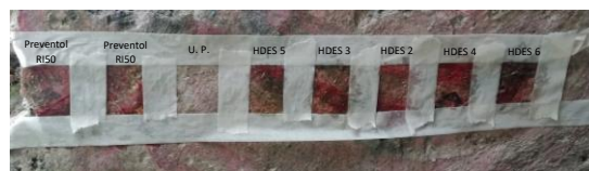
Fig. 5 Application of HDESs during conservative treatment of "Déesis" in Motta San Giovanni (Reggio Calabria).
