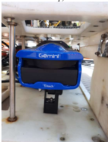
Fig. 3: Gemini 720is acoustic camera, positioned at the front of the ROV (S. Fontaine, Inrap)
