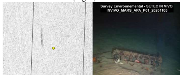
Fig.1: Anomaly identified on the low acoustic data of the initial survey and its visual correspondence during the Rov survey of Setec In Vivo.
