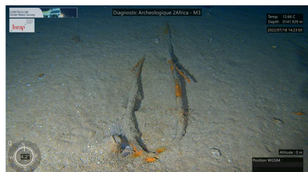
E. Cable loop partially buried
