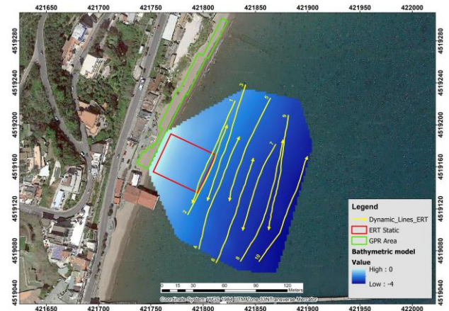
Fig. 3. Layout of the GPR and static ERT grids long with the dynamic 2D ERT lines on a Google Earth satellite image.
