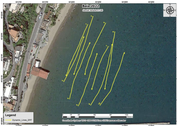
Fig. 6. Layout of dynamic ERT lines superimposed on a Google Earth satellite image of the study area.
