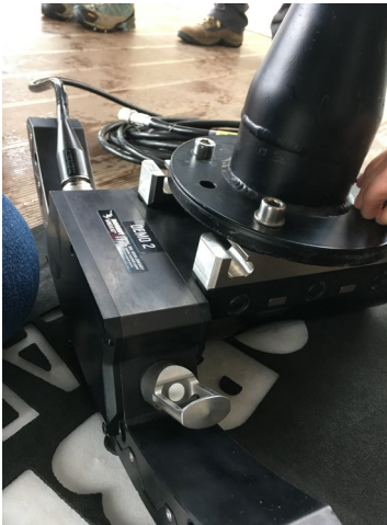
Fig.4. Sonar head of the WINGHEAD i77h MBES system
