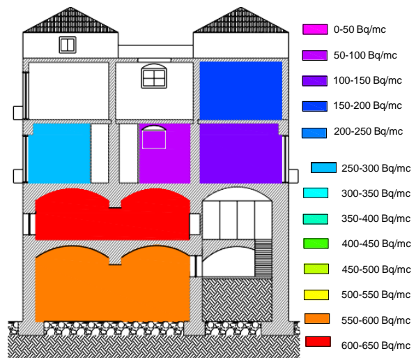
Fig.3. Graphical representation of the measurements of indoor radon activity concentrations ranged in classes.
