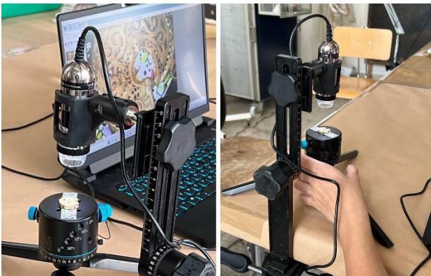
Fig. 3. The image-based acquisition system assembled to employ a USB microscope for photogrammetric purposes.
