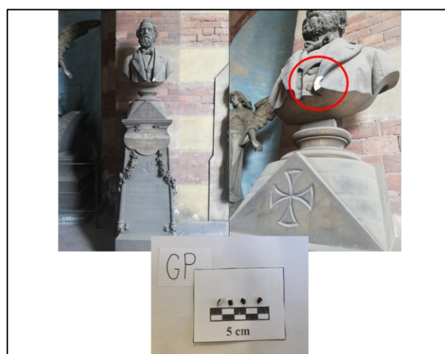
Fig. 3. Bust on pillar funerary monument (sample GP) with the indication of the area (red circle) from which the collected black crusts were detached.
