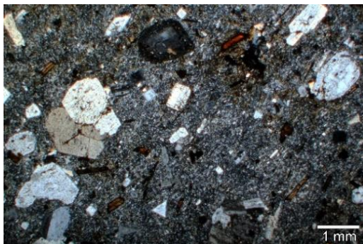
Fig. 5 – AD_79, Trachyte from M. Oliveto (PLM – crossed polars).
