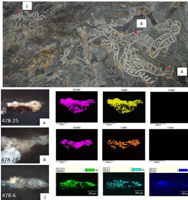
Figure 2: SEM-EDS mapping of samples taken from the snake motif at La Candelaria cave.
