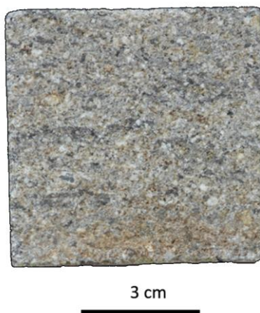
Fig. 1. Example of a Peperino stone used in this project as a sample.
