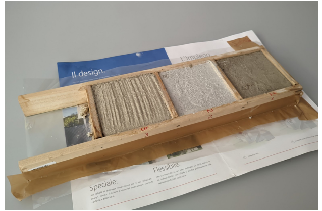
Fig. 3. Prepared samples in their wooden formwork. The variations in color between samples are due to differences in material composition.
