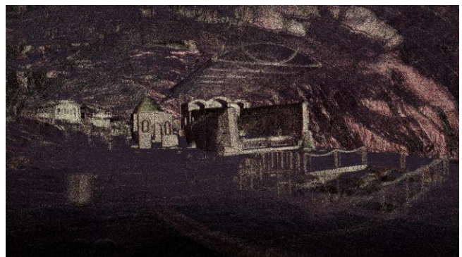
Fig. 2 Integrated point cloud of the Grotta di San Michele Arcangelo. Author's elaboration.
