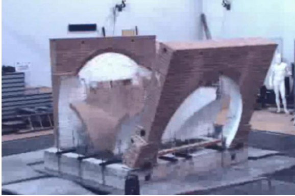
Fig. 4. Complete activation of collapse mechanism (time t = 6.0 s).
