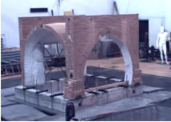
Fig. 1. The masonry structure on the shaking table at the beginning of the test.
