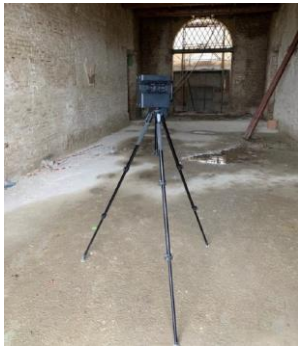
Fig. 2. Survey with Matterport Pro2.
