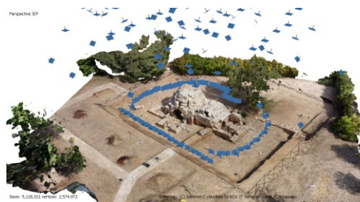
Figure 2: Photogrammetric 3D model and relative acquisition scheme
