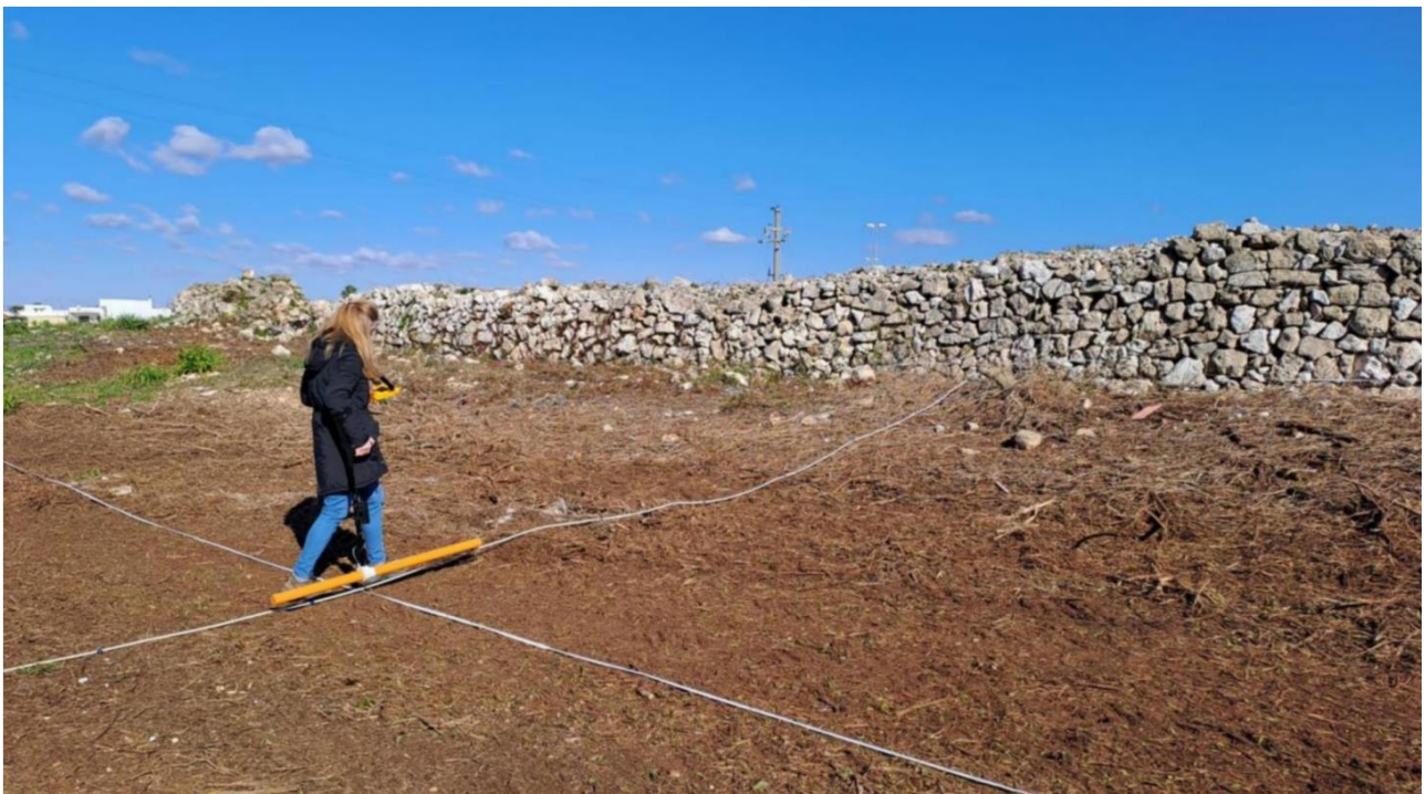
Fig. 2. The electromagnetometer CMD mini-explorer by GF instruments. It is composed by 3 receiving coils that allow to obtain information in n. 3 depth ranges. As the distance between the transmitting coil and the receiving coil increases, the depth of investigation increases.
