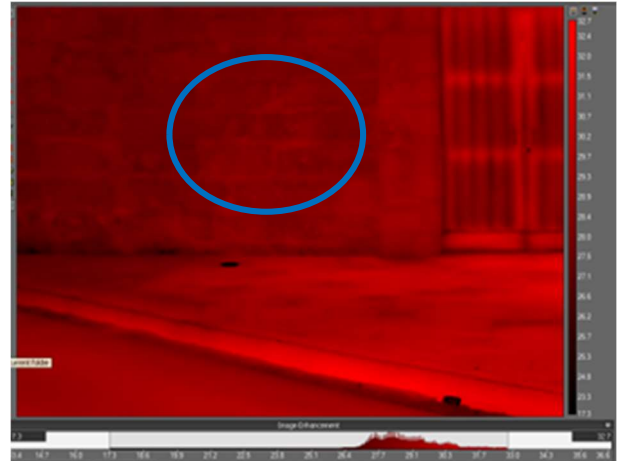
Fig. 7. Hidden structure at the left side of the church main entrance
