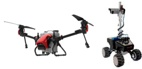
Fig. 4. Two examples of commercial drones for agriculture. (a) is the XAG V40 (4.2gal / 15L), a drone with a 15 liters tank, (b) is VINBOT, an all-terrain autonomous mobile robot with a set of sensors capable of capturing data about water status, production, vegetable development or grape composition.
