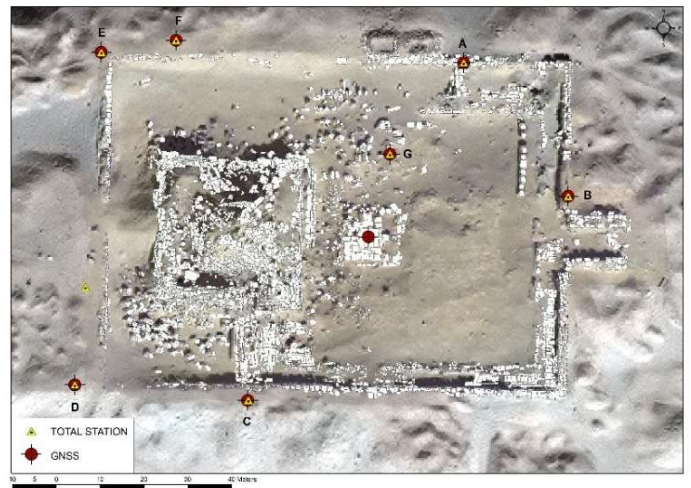
Fig. 4. The benchmarks around the excavation area
