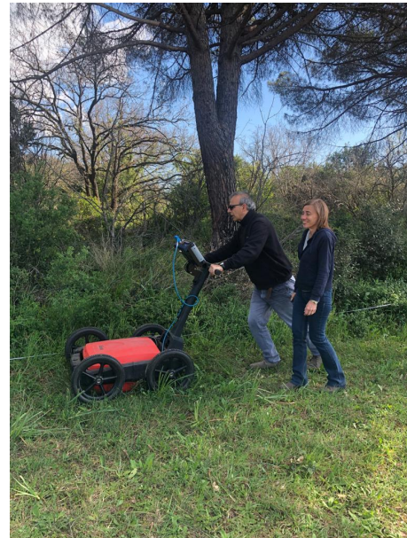
Fig. 2. GPR data acquisition in Banditaccia
