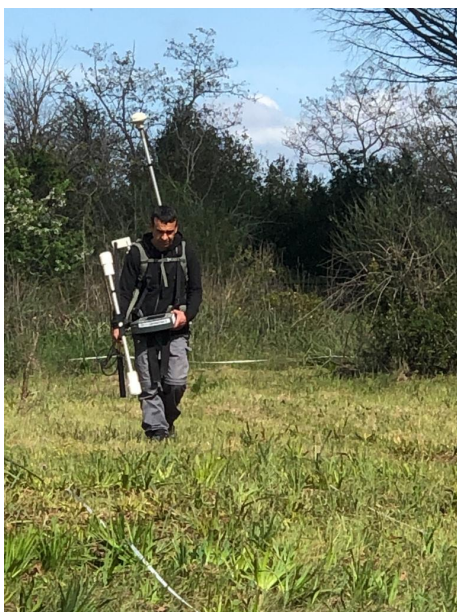
Fig. 3. Magnetometric data acquisition in Banditaccia
