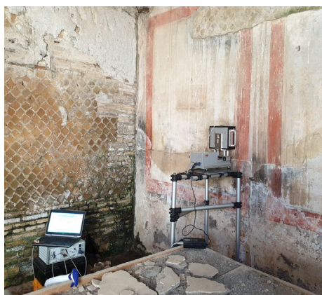
Figure 2. Setup of the NMR-MOUSE when measuring a depth profile into a painted wall in the Mitreo di Lucrezio Menandro. The sensor with a strong magnet rests on a displacement stage on top of a scaffold close to the wall for point-by-point acquisition of a depth profile.
