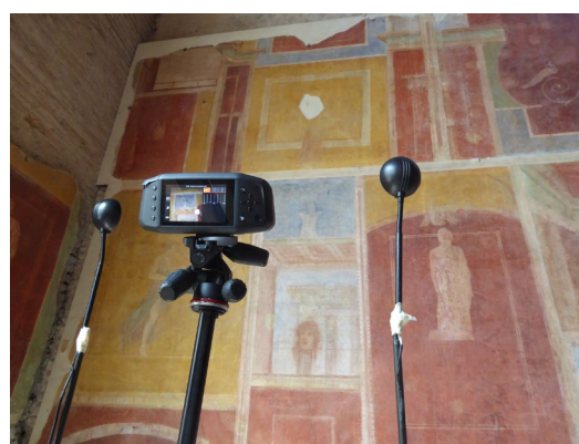
Figure 4. The compact HSI camera during the measurements campaign of the paintings in the main room of the Giove and Ganymede house.
