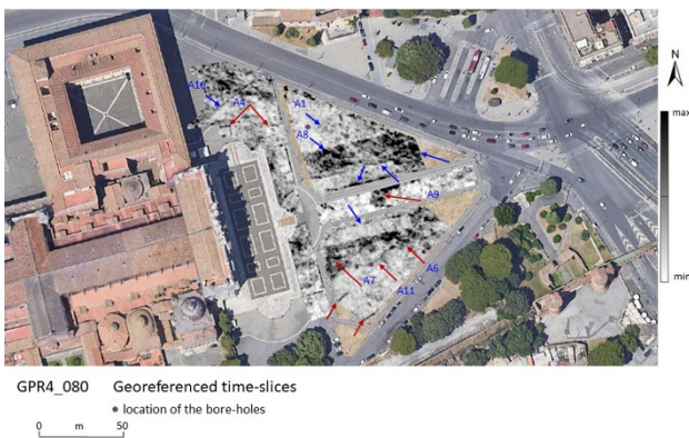
Fig.2 – S. Giovanni in Laterano square. GPR time-slices at the estimated depth of 0.80 m.
