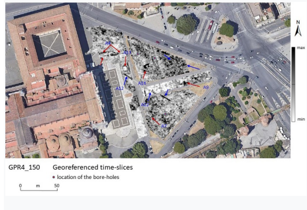
Fig. 3 – S. Giovanni in Laterano square. GPR time-slices at the estimated depth of 1.50 m.
