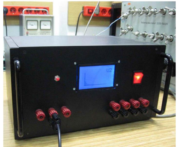
Fig. 4[3]. A stochastic instrument proposed in [3] for stochastic measurement of harmonics at low signal-to-noise ratio.
