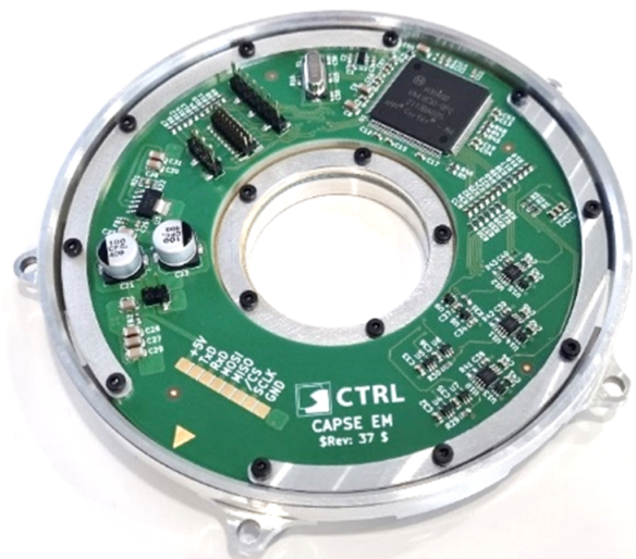
Fig. 1. CAPSE sensor prototype with embedded RadHard microcontroller.
