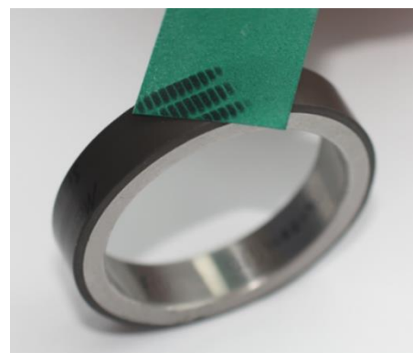
Fig. 3. Magnetisation pattern on a pole ring (Image source: Sensitec GmbH).
