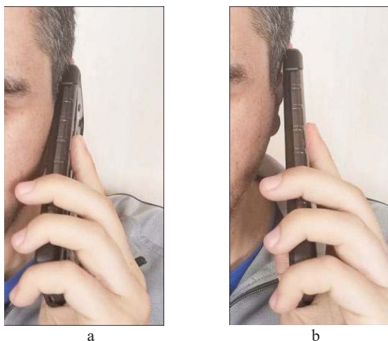
Fig. 4. Huawei P20 Pro phone with a protective case in the cheek position (a) and the tilt position (b) towards the user's head
