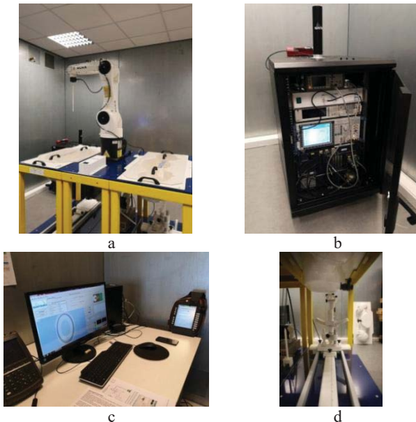
Fig. 1. The SATIMO-COMOSAR system used for SAR measurements: (a) KOMOSAR test bench and KUKA robot, (b) signal generator Rohde & Schwarz CMU 200, (c) computing unit with OPENSAR software installed for testing system control (d) the fastening system used to secure the measuring equipment
