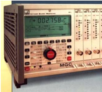
Figure 1: Measurement amplifier MGC
