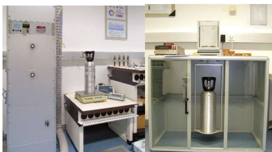
Figure 12: Filling station and comparative balance
