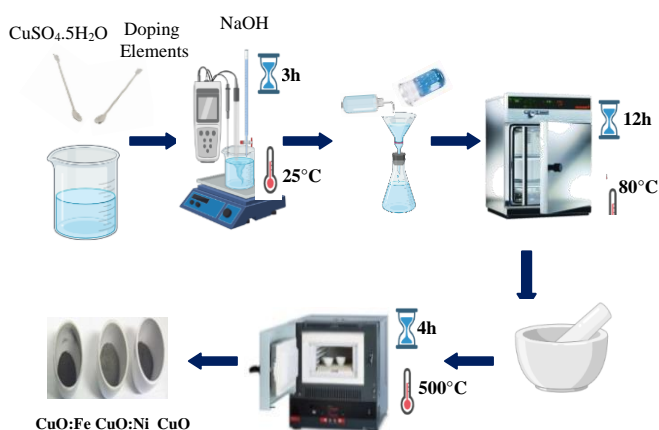
Figure 2: Schematic representation of the synthesis procedure by co-precipitation of undoped and -doped CuO NPs
