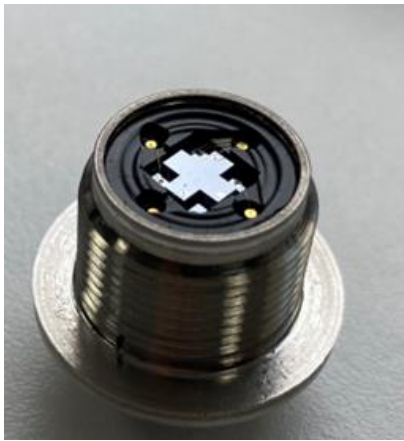
Fig. 2. Silicon die packaged in a glass-to-metal seal
