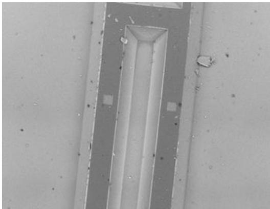
Fig. 5: REM Image of a MEMS-SOIMT Sample Fragment with a frame of a regular shape
