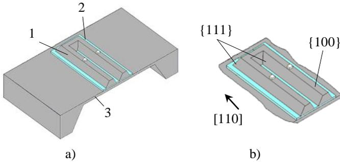
Fig. 1: Cross-Section of a Microelectromechanical Piezoresistive Sensor Based on SOI structure: (a) 1 – integral monolithic tensoframe, 2 – thin dielectric layer, 3 – membrane; (b) crystallographic orientation of a tensoframe after anisotropic chemical etching of silicon (100)
