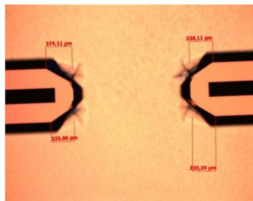
Fig. 3: Photo of tensoframe sample fragments with the frame undercut bias equal 38,25  $\mu\text{m}$
