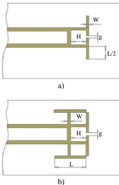
Fig. 2: Fragments with Angle Compensators for ACE Process: with Configuration 1 (a) and Configuration 2 (b)
