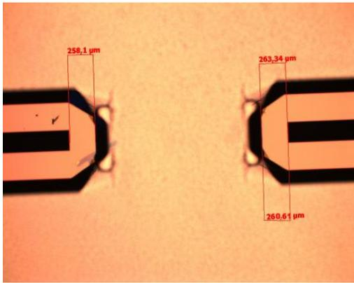
Fig. 4: Photo of tensoframe sample fragments with the frame undercut bias equal 2,73 μm
