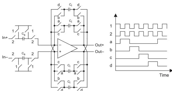
**Figure 4.** Schematic of the single operational amplifier resonator used
