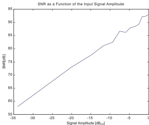
Figure 6. SNR as a function of the signal amplitude of the proposed A/D converter
