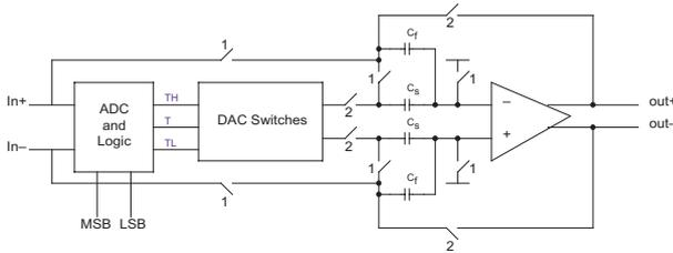
**Figure 3.** Schematic of the 1.5 bit pipeline stage
